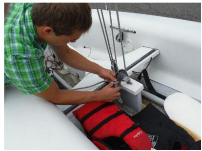
6. Ask your crew person to hold the boom while you loosen the main halyard (tied to the outhaul, aft end of the boom) so the boom will not drop into the boat.
