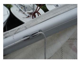
6. Untile the main halyard from where you secured it and make sure that the end running down the boom side of the mast is not twisted or fouled.
