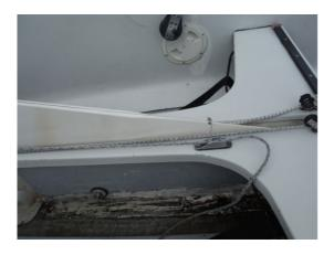
3. If there is water in the boat, undo the drain plug and lift the boat at the shrouds or bow to drain it.
