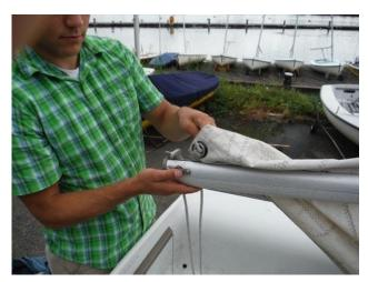
5. Run the outhaul up the boom to the jam cleat near the mast. Push the outhaul into the cleat and secure it with a figure 8 knot.
