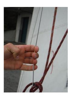
5. Run the jib sheets through the blocks and tie a figure 8 knot at the end of each.
