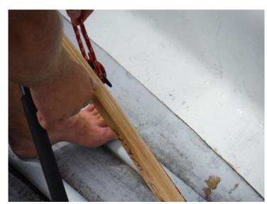
Your rudder should also be secured to the boat with a lanyard. The setup may vary from boat to boat. Simply check – if you rudder came off the pintles, would it float away or be attached to the boat?
