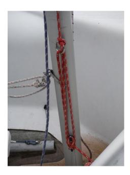
3. Pass the Cunningham through the small grommet above the tack and tighten it down in the mast jam cleat.
