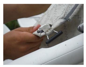
2. Feed the clew (rear corner) of the sail into the slot, starting at the tack end (near the mast); pull it down to the stern end of the boom.
