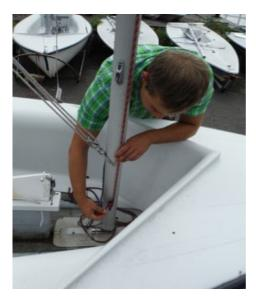
7. Tie the halyard's ends together so that it does not get loose and sky at the top of the mast. The ring and a wet halyard together can be enough weight to pull the loose end up out of reach
